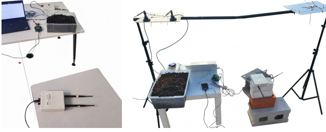
(a) Deployment 1: receiver at soil height. (b) Deployment 2: elevated receiver, with two tested transmitter configurations.
